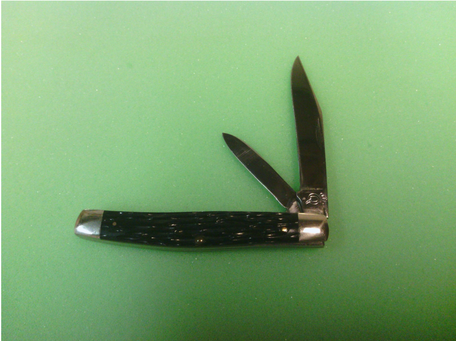
Figure 2. #2, Queen, serpentine jack, 2 blade, rough black imitation bone handles, brass liners, NS bolsters, no etch, Big Q tang stamp, 3-1/4"
