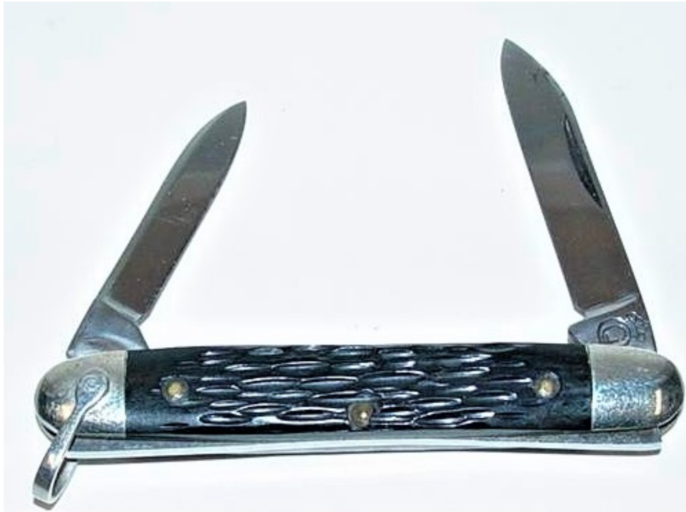
Figure 4. #7, Queen, senator pen with bale, 2 blade, rough black imitation bone handles, brass liners, NS bolsters, no etch, big Q tang stamp, 2-1/2"
