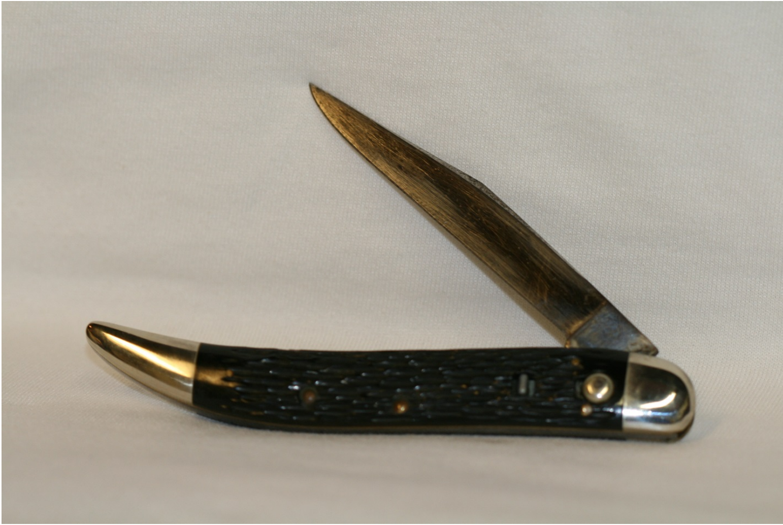
Figure 5. #25, Queen, Jet push button w/safety lock, 1 blade, rough black imitation bone handles, brass liners, NS bolsters, no etch, big Q tang stamp, 5." (Not really considered "Rough Black," shown only to show similarities in delrin handle material. Collected vigorously in its own right)
